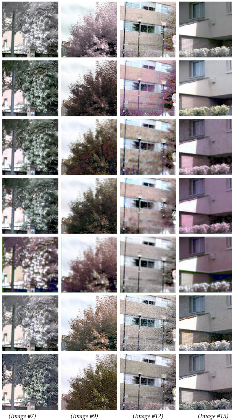
Figure 6. Four samples from the average and worst results (see Table 2). (1st row) X images (RGB + N). (2nd row) Y (ground truth). (3rd row) Results from CDNet. (4th row) Results from ENDENet. (5th row) Results obtained with SRCNN ([30]). (6th row) Results obtained with ref. [21]. (7th row) Results obtained with ref. [20]. The image numbers correspond to the values presented in Table 2.
