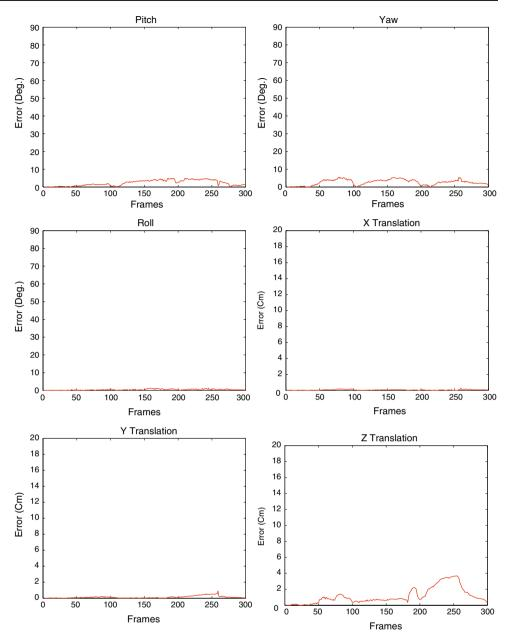
returns a 3D rigid displacement that directly quantifies the monocular tracker accuracy.
