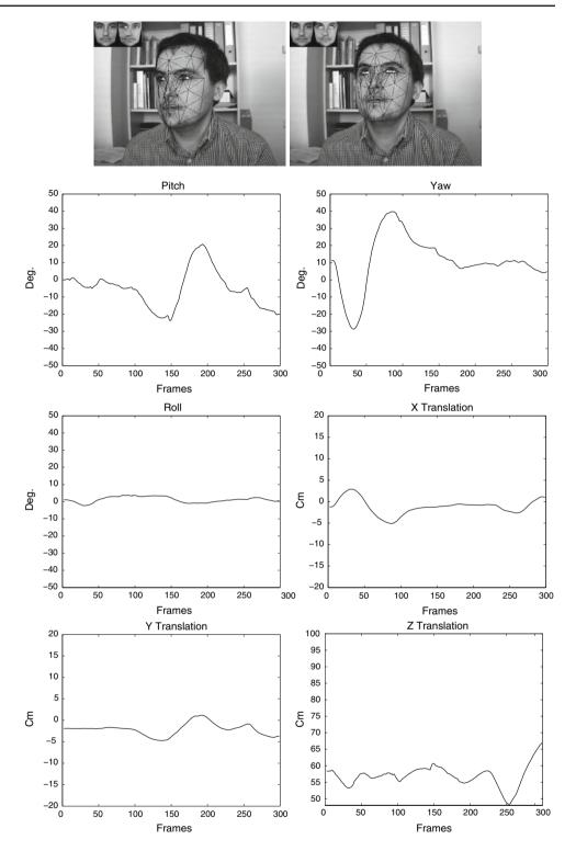
(1) the proposed appearance-based approach (Sect. 4) using the monocular sequence provided by the right camera, and(2) the 3D face motions computed by 3D registration of 3D facial data in different frames. Recall that the 3D rigid displacement that align two facial clouds obtained at two different frames is equivalent to the performed 3D head motion between these two frames.
