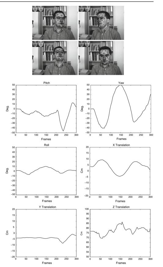
Fig. 8 The estimated 3D head pose parameters associated with the third video. Only frames 38, 167, 247, and 283 are shown
