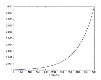
Fig. 3 A sliding exponential envelope having  $\alpha$  equal to 0.01. The current frame/time is 500. The vertical coordinate corresponds to the blending weight
