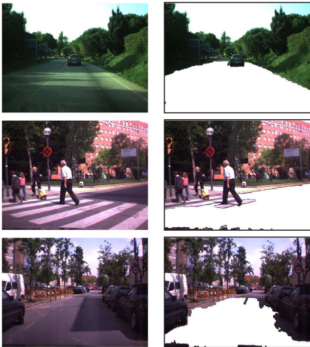
Fig. 9. Segmentation results associated with extreme light variations. The left column is the original image that covers the nearest 80 m ahead of the vehicle. The right column shows in white the corresponding segmented road.
