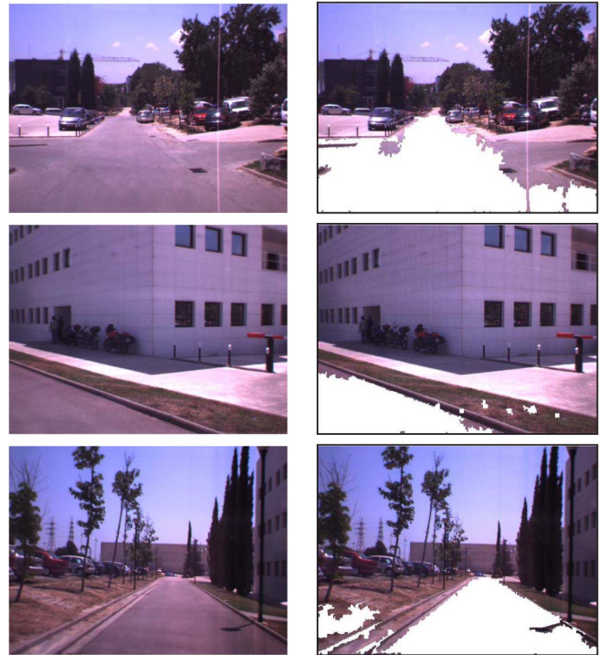
Fig. 10. Challenging road sequence. The left column shows the original image. The right column shows in white the corresponding segmented road.
