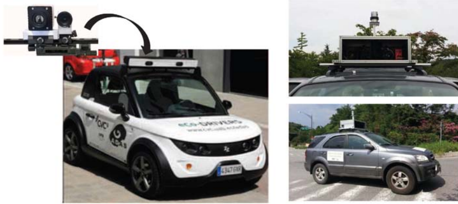
Fig. 4. Acquisition systems (cross-spectral imaging on the top): (left) Electric vehicle from the Computer Vision Center (Barcelona, Spain) [5] (CVC video sequences); (right) Car from the Korea Advanced Institute of Science and Technology (Seoul, Korea) [29] (KAIST video sequences).
