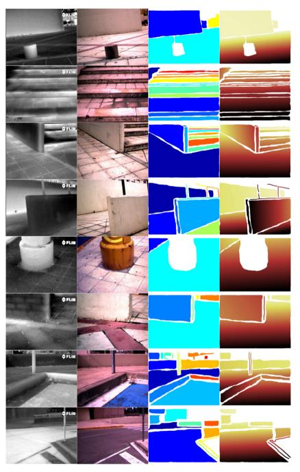
**Fig. 7.** Examples of evaluation data set; each column corresponds to: (1st)  $I_{LWIR}$  images; (2nd)  $I_{VS}$  images; (3rd) maps of planar regions; and (4th) synthesized disparity maps used as ground truth for evaluating the proposed approach.
