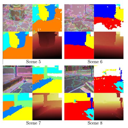
**Fig. 9.** Experimental results from different stages of the proposed approach; in each scene the illustrations correspond to: (*top-left*) support region *R*; (*top-right*) planar hypotheses Π; (*bottom-left*) labeled regions from graph cuts; and (*bottom-right*) final disparity map.
