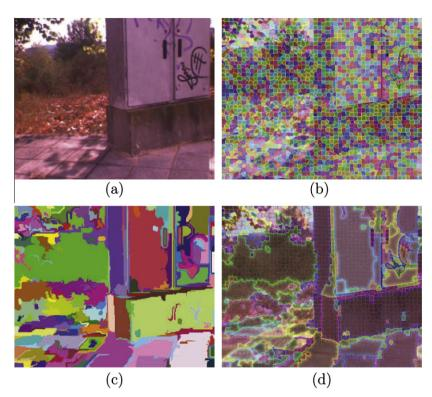
**Fig. 3.** Illustration of the support region segmentation: (a) original  $I_{VS}$ ; (b) superpixels (S) obtained from Levinshtein et al. (2009); (c) perceptual regions (P) from Felzenszwalb and Huttenlocher (2004); and (d) support regions (R) obtained by fusing (b) and (c).
