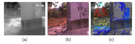
Fig. 2. Inputs and output images of first stage: (a) rectified infrared image ILWIR; (b) rectified visible image IVS; and (c) initial sparse disparity map Dmap\_0.
