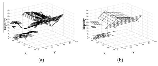
Fig. 5. Planar hypotheses simplification: (a) original set of planar hypotheses from the segmentation presented in Fig. 3 (179 planes) and (b) planar hypotheses resulting after four iterations of the postprocessing stage (14 planes).
