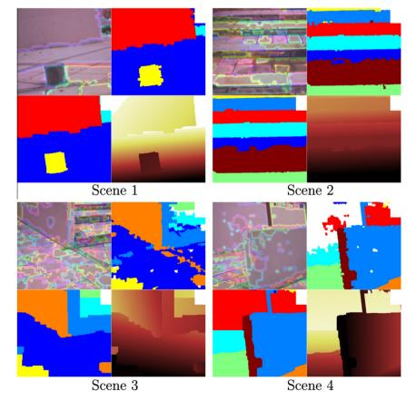
**Fig. 8.** Experimental results from different stages of the proposed approach; in each scene the illustrations correspond to: (*top-left*) support region *R*; (*top-right*) planar hypotheses Π; (*bottom-left*) labeled regions from graph cuts; and (*bottom-right*) final disparity map.
