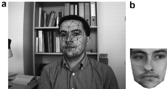
Fig. 1. (a) An input image with correct adaptation and (b) the corresponding shape-free facial texture map.
