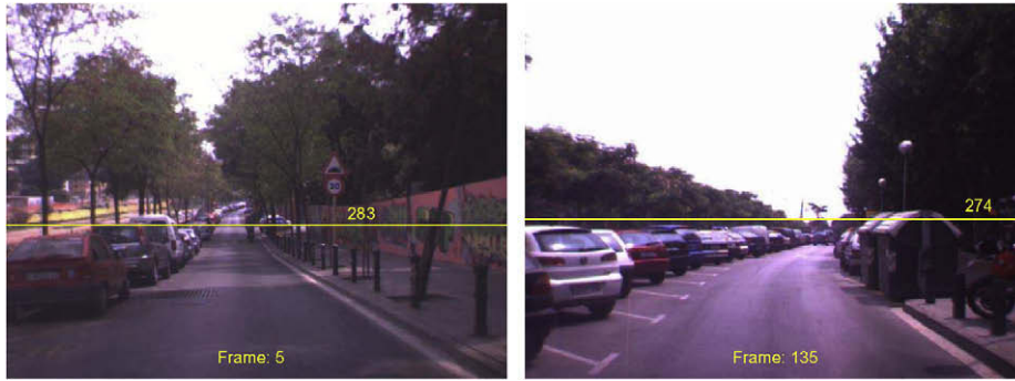
Fig. 12. Estimated horizon line (white line) in frames acquired in a narrow urban road. The robustness of the proposed technique can be qualitatively appreciated, in spite of the car-cluttered street.
