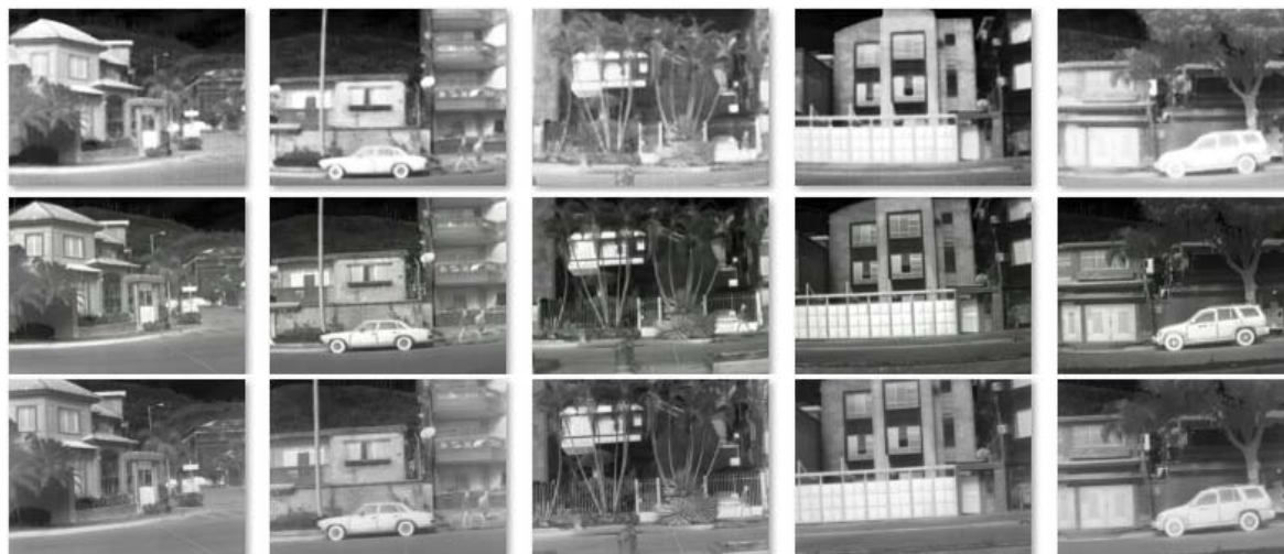
Figure 7: Examples of thermal images used for training. ( top ) LR images from Axis Domo P1290. ( middle ) MR images from Axis Q2901-E. ( bottom ) HR images from FC-6320 FLIR.
