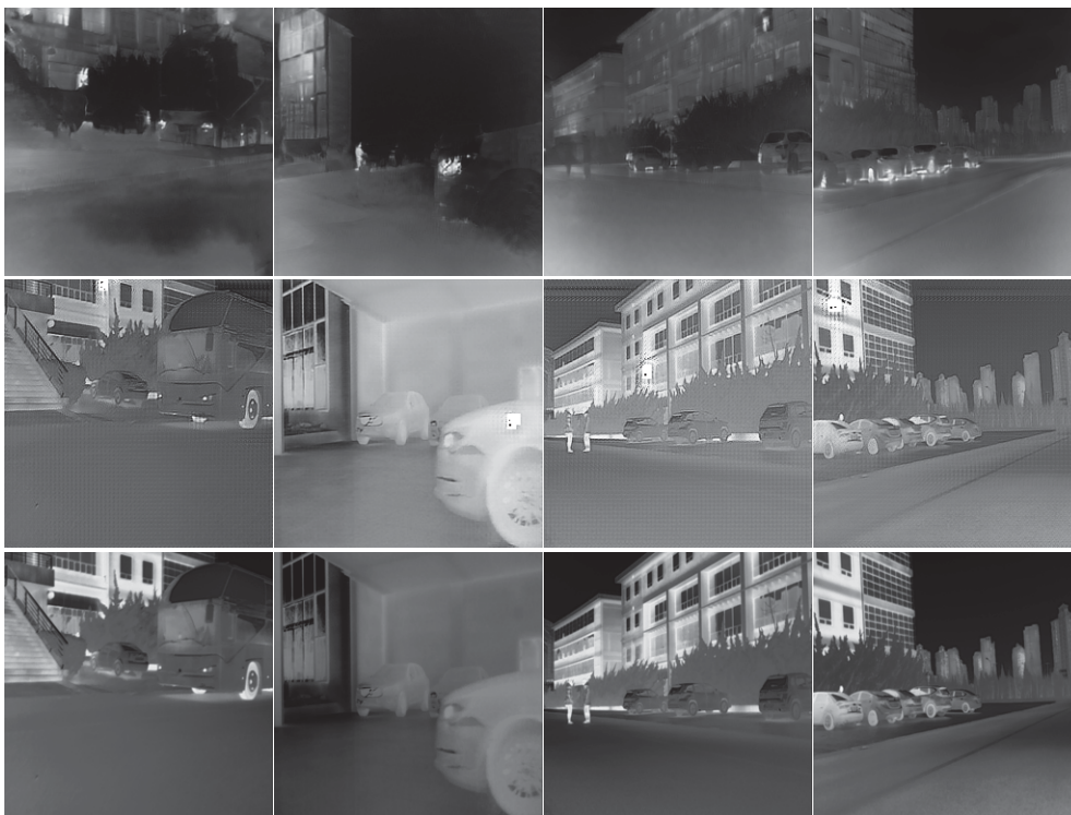
Figure 2: Experimental results: ( 1st. row ) results with state of the art technique (Zhu et al., 2017); ( 2nd. row ) results from the proposed approach; ( 3rd. row ) ground truth images from M3FD and Thermal Stereo datasets.
