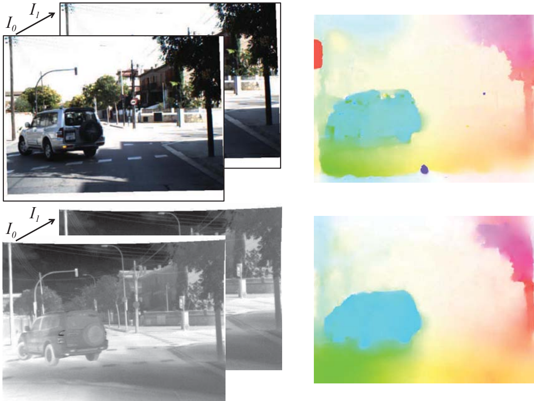
Figure 2: (left) Two pairs of cross-spectral images (VS and LWIR). (right) Dense flow fields used for the correspondence search.
