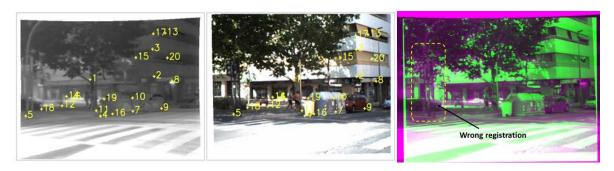
Fig. 1. Registration of LWIR and VS images. (left) LWIR image with the set of keypoints (20 points); (middle) VS image with the corresponding keypoints (20 points); (right) Registration result obtained by minimizing MSE (this figure is best viewed in color).
