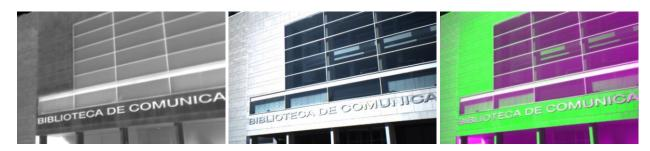
Fig. 3. (left) Input LWIR image. (middle) Input VS image. (right) Result from the MI Registration (input images are overlapped using different colours to appreciate the results).
