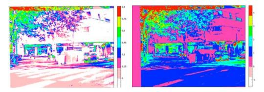
Fig. 4. (left) NDVI, using LWIR instead of NIR. (right) RVI, using LWIR instead of NIR (this figure is best viewed in color).
