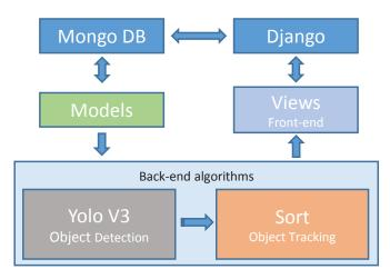
Fig. 1: General scheme of software architecture.
