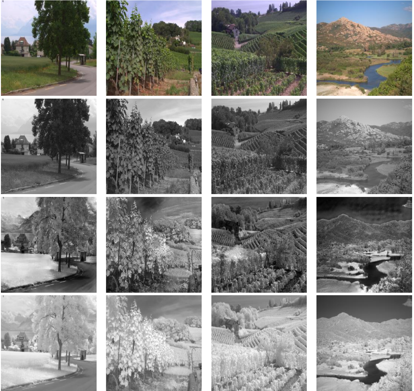
Figure 2. Illustration of NIR images obtained by the proposed CycleGAN, which are later on used to estimate the corresponding NDVI indexes. (1st.row) RGB images. (2nd.row) Gray scale image used as input into the CycleGAN. (3rd.row) Estimated NIR images. (4th.row) Ground truth NIR images. Images from [3], country , field and mountain categories.
