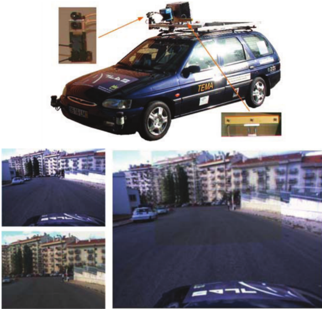
Fig. 1. The Atlascar robotic platform with several onboard cameras (top) ( http://atlas.web.ua.pt ). Onboard images taken with two cameras from a typical road scene. Source image (bottom-left-top), Target image (bottom-left-bottom); the mosaic of both which shows a clear difference in colors (bottom-right); .
