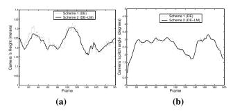
Fig. 5. Camera height and orientation computed by the proposed tracking schemes
