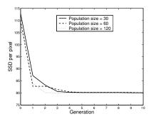
Fig. 6. The evolution of the best registration error obtained by the Differential Evolution algorithm associated with the first stereo pair.
