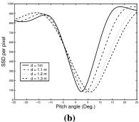
Fig. 10. The registration error as a function of the camera pose parameters. (a) depicts the error as a function of the camera height with a fixed orientation. (b) depicts the error as a function of the camera pitch angle associated with four different camera heights.
