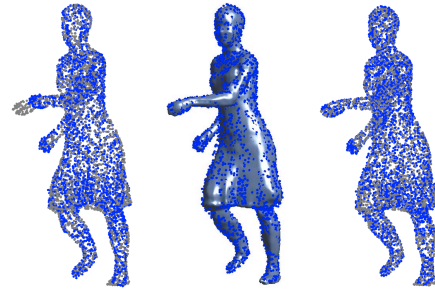
Figure 7. ICP approach in ( left ) easily gets stuck in a local minima, while using interfaces leads to the global minimum ( right ).
