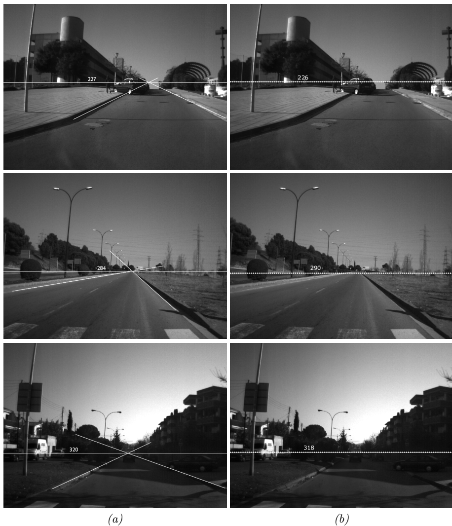
Fig. 5. Illustrations of vanishing lines manually estimated (a) and automatically computed by the proposed technique (b). (top) Uphill driving illustration. (middle) Flat road. (bottom) Downhill driving scene.
