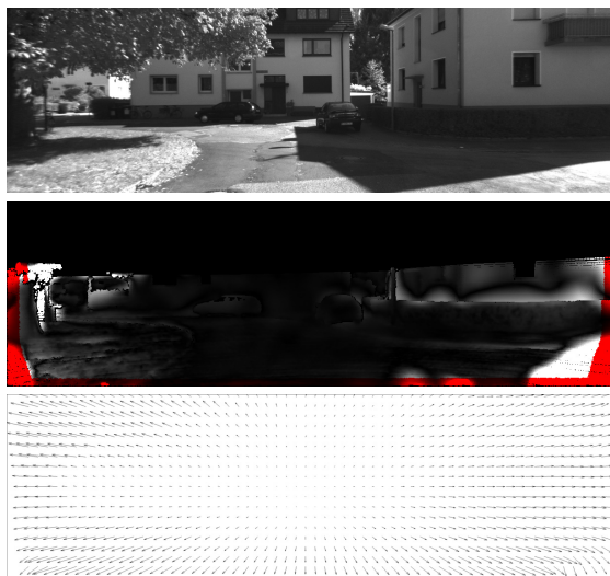
Fig. 2. Results for a pair of images; ( top ) 1 st image of the pair; ( middle ) error map; and ( bottom ) computed flow field.
