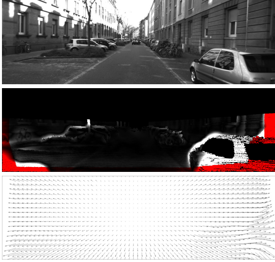
Fig. 3. Results for a pair of images; ( top ) 1 st image of the pair; ( middle ) error map; and ( bottom ) computed flow field.
