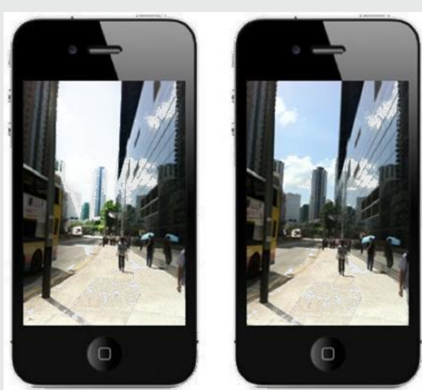
LDR image of HDR scene, without using tone-mapping operator (left) and using one (right).
